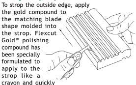
polish hardened steels. The bevel of the tool should be placed as flat against the strop as possible. The tool is then pulled away from the edge to avoid digging into the strop. If the angle of the bevel against the strop is too high, it will round prematurely. If it is too low, the edge will not be properly abraded.
