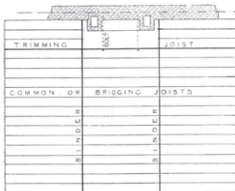
Fig. 325.—Plan of Binder or Double Floor.
