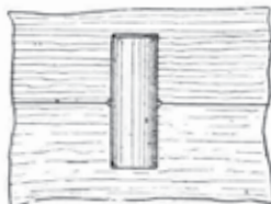
Fig. 295.—Dowelled Joint Correctly Made.
