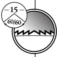
**15-60/60:** Old-world French combination blade. This is also a traditional pattern, but it seems to spark the most controversy. Because the blade features teeth that appear to 'face' each other, this blade can cut with different characteristics depending on how you hold it. For some, this can be infuriating; for others, it's a joy to use. In the workshop here at Gramercy Tools, it's a house favorite.
