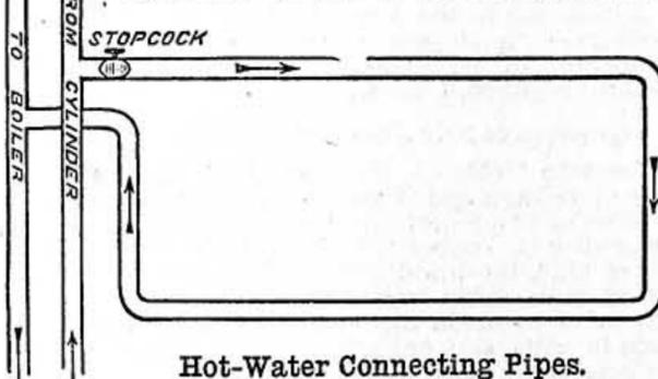
**Hot-Water Connecting Pipes.**
