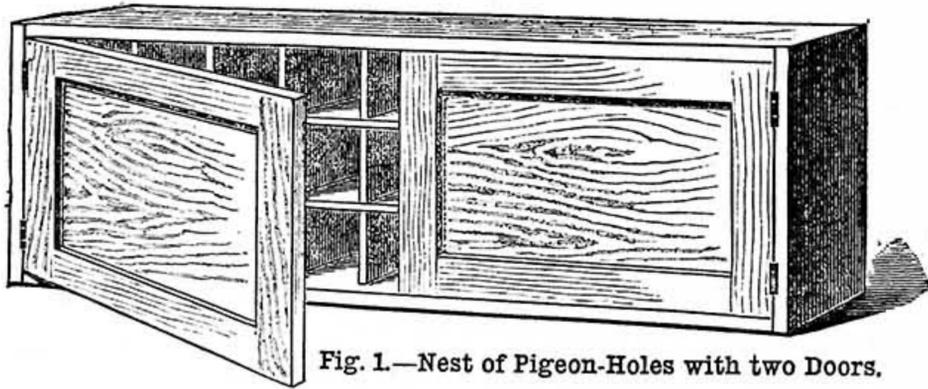
Fig. 1.—Nest of Pigeon-Holes with two Doors.
