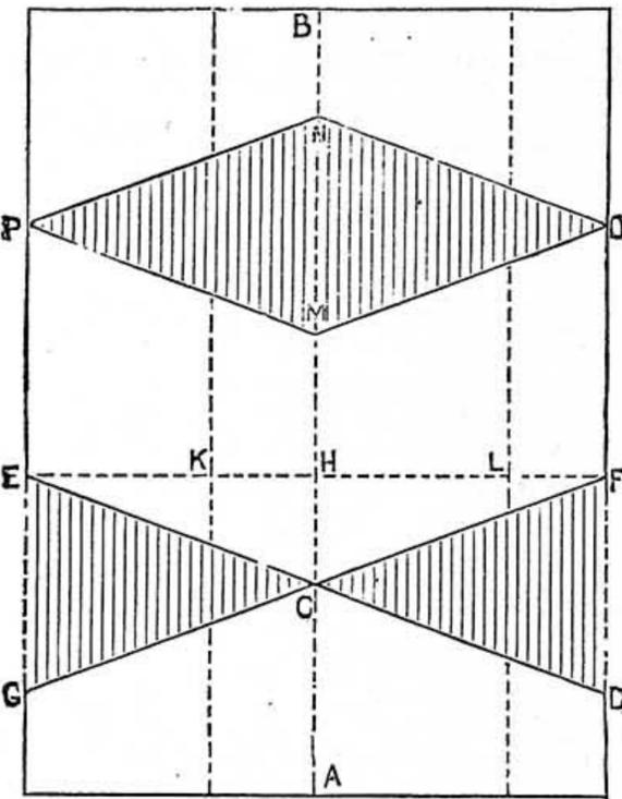
Pattern on Flat Surface for Rain-Water Down Pipe to go over Return Plinth, with 3 in. Projection and 3 in. Rise.
