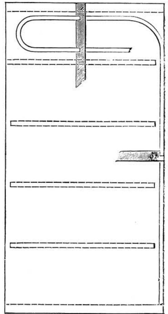
Fig. 4.—End of Nest showing Groove and Rebate on Front Edge. Dotted Lines show Position of Shelves.
